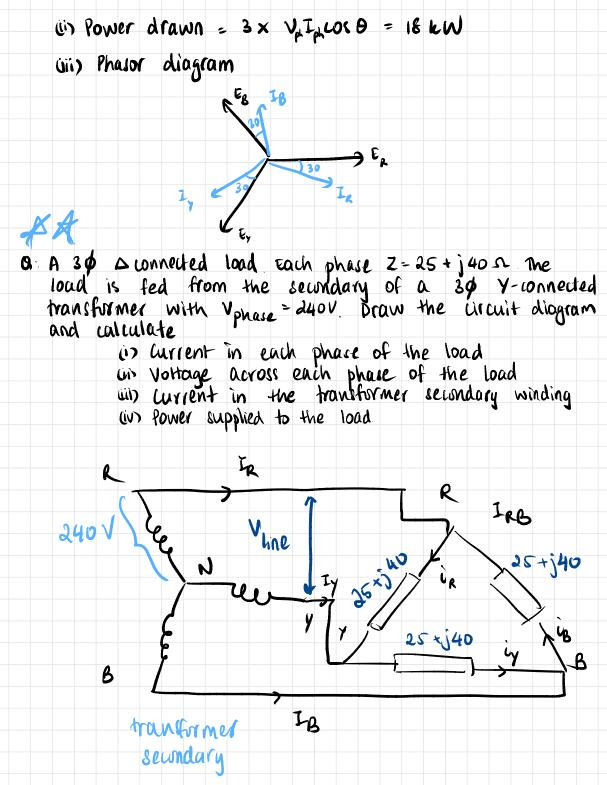
line voltage of Y transformer = phase voltage of S wad
