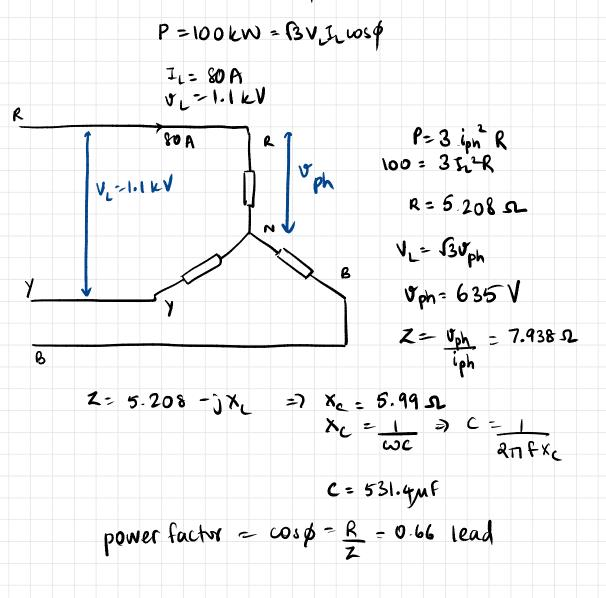
G A balanied 3\$\$ star-connected load is supplied with a
