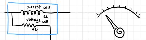
• two coils: fixed coil  $\rightarrow$  gives magnetic flux voltage coil  $\rightarrow$  indicated the power
