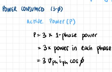
$$P_{3p} = 3 \times \frac{V_{L} I_{L} \cos \phi}{(3)}$$
