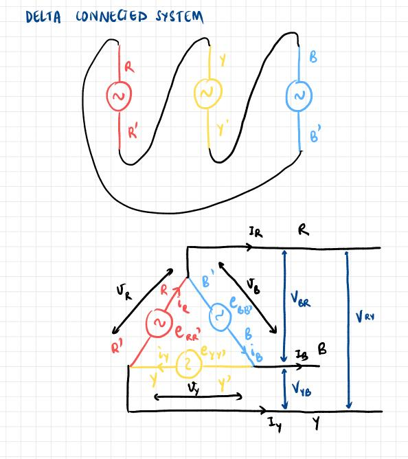
· In D connection, second terminal of first coil is connected to the first terminal of the second coil, and so on
