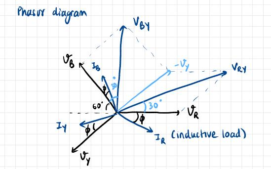
Power measured by  $W_1 = V_{RY} T_R \cos(angle b/w V_{RY} & T_R)$   $= (V_R - V_Y) T_R \cos(angle)$   $W_1 = V_{RY} T_R \cos(30 + \phi)$   $W_1 = V_L T_L \cos(30 + \phi)$ Power measured by  $W_2 = V_{BY} T_Y \cos(angle b/w V_{BY} & T_Y)$   $= V_{BY} T_Y \cos(30 - \phi)$  $W_2 = V_L T_L \cos(30 - \phi)$
